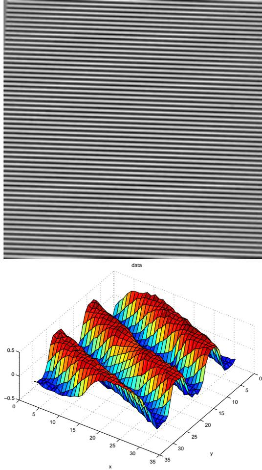
**Figure 5:** The intensity difference image generated by the highest order band pattern projected onto a planar surface by the Structured Light System. Below this is a plot of the values in a small patch
