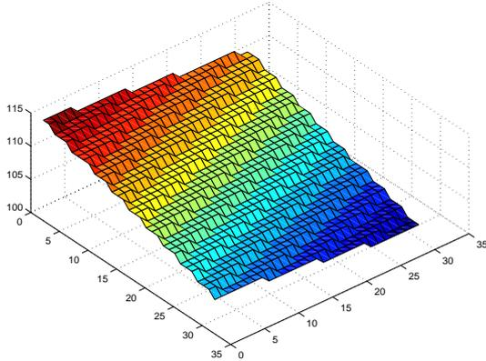
**Figure 2:** The stripe ids in a  $36 \times 36$  data patch from a plane, plotted as functions of image plane coordinates. Note the step effect due to the discretisation of the projector emitter plane coordinates.
