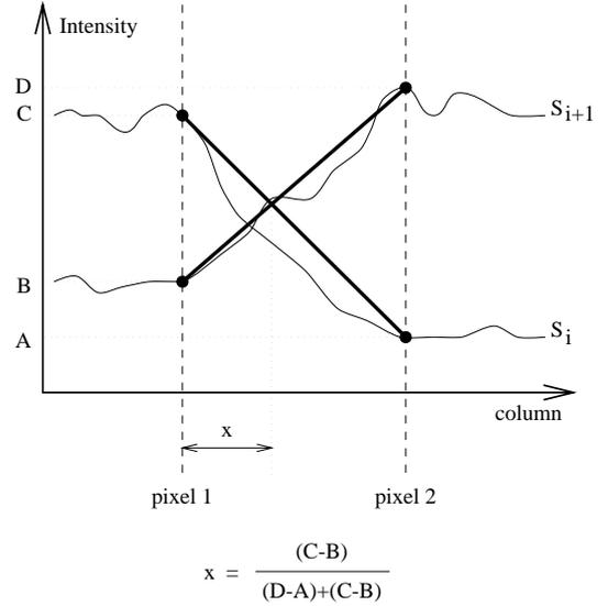
**Figure 3:** The operator used for locating zero-crossings in an intensity differential pair. It is applied between two pixels where the difference image changes sign.
