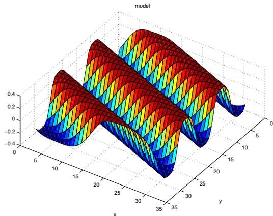
**Figure 6:** The sinusoidal model fitted to the intensity difference image in Figure 5.
