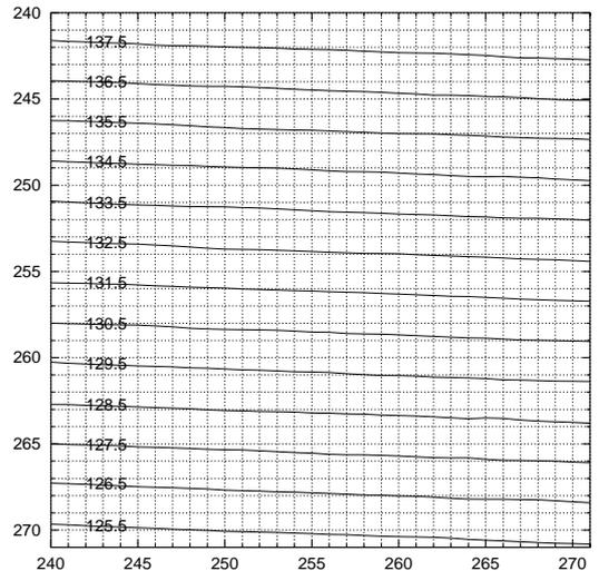
**Figure 4:** Stripe boundaries detected in the central  $32 \times 32$  patch of data from a planar surface. The grid connects pixel centres. A boundary's label indicates its the projector emitter plane coordinate.
