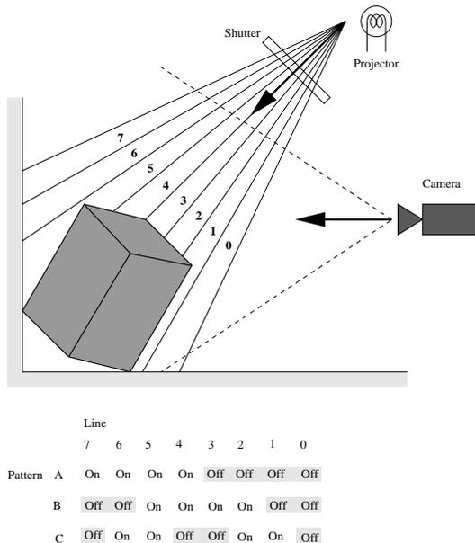
**Figure 1:** A model of a temporally encoded structured light system showing how the projector emitter plane stripes are encoded over the sequence of images. In the illustration, 8 stripes (labelled 0...7) are encoded by three images (A, B, C).
