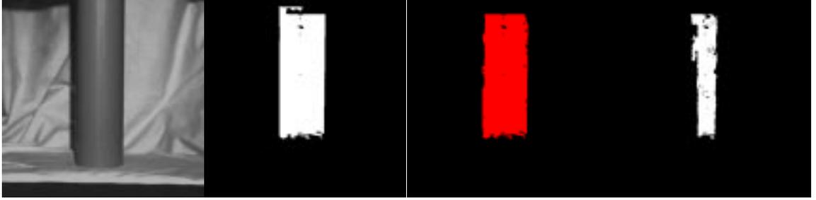
**Figure 2: Example of cylindrical region extraction. From left to right: An image of a scene containing a piece of pipe; A mask indicating the largest connected region of parabolic points; The largest cylindrical region extracted by region growing; The largest cylindrical region extracted by Bayesian classification.**
