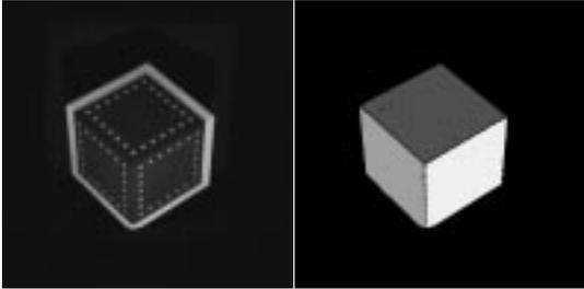
Figure 1: The image on the right shows the connected planar regions identified in 3D data taken from the scene on the left.
