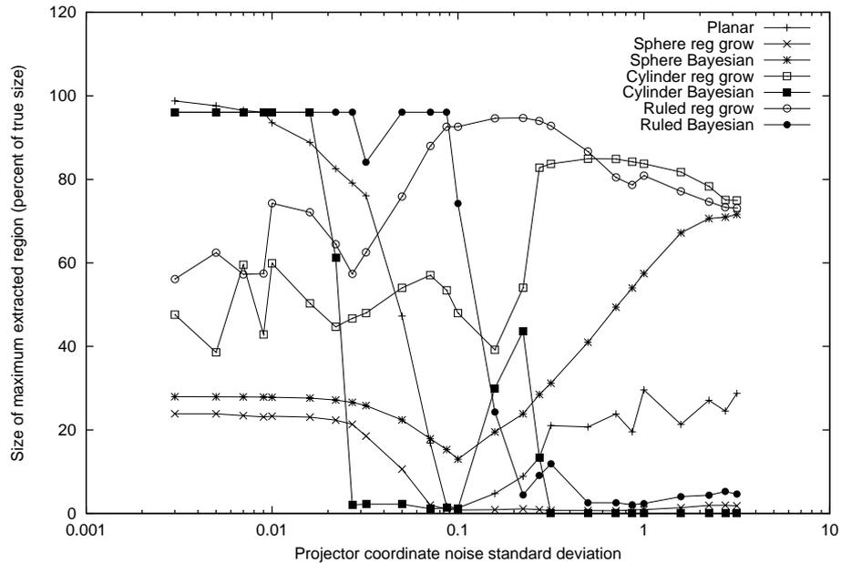
**Figure 3: The size of the extracted regions, as a percentage of the true size, for the Monte-Carlo simulations of the methods.**
